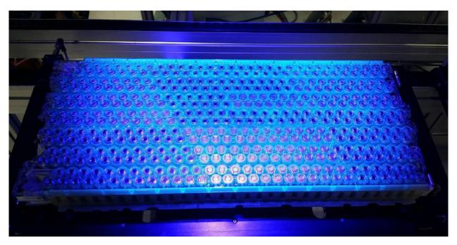
In this exercise you will study a data set on battery capacity collected by researchers from AAU Energy. The batteries were kept at three different temperatures. The capacity loss Q (in percentage of initial capacity) is the response variable. We are interested in the effect on the response of the temperature and the efficient number of charge cycles FEC that the battery had been exposed to.
