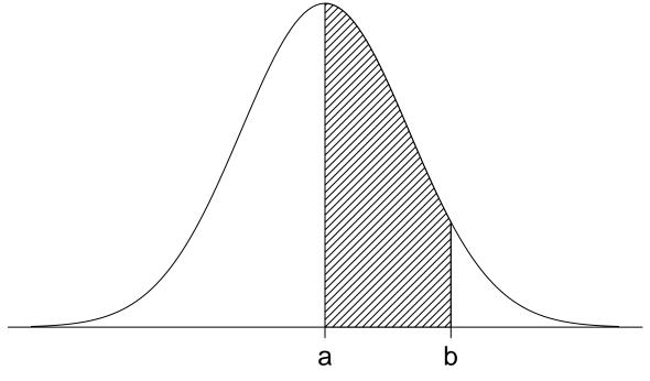
• The area under the graph of the probability density function between a and b is equal to the probability of an observation in this interval.
