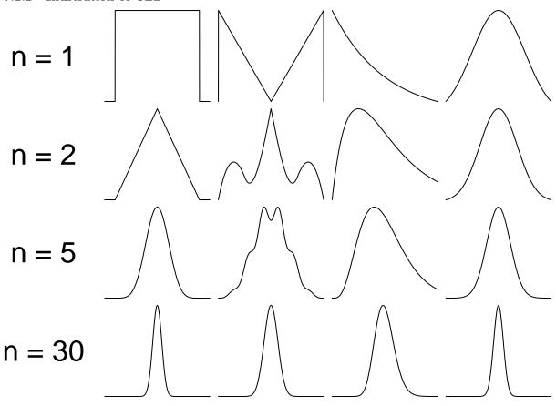
• Four different population distibutions (n=1) of y and corresponding sampling distributions of  $\bar{y}$  for different sample sizes. As n increases the sampling distributions become narrower and more bell-shaped.
